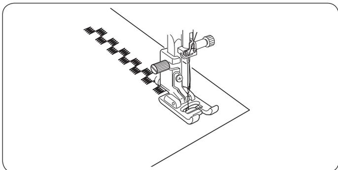
For a delicate appearance on fabric such as chiffon, use a single layer with a tear-away backing, if necessary.
